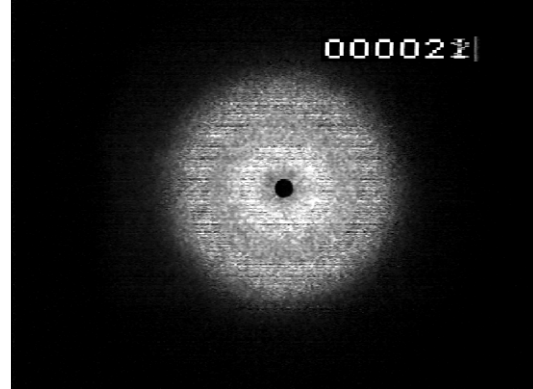
Fig. 9. Unpolarised light scattering pattern obtained at 22.5 °C for 4 mW cm -2 .
